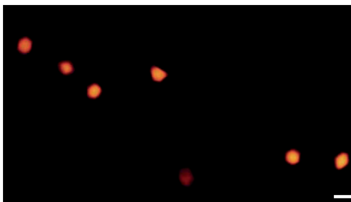
Figure 4.4: Dispersible rhombic dodecahedron like particles. Confocal microscopy image of rhombic dodecahedron type PMMA particles in CHB. Although it is difficult to observe the rhombic dodecahedron shape from the image it clearly shows that the particles are not spherical in shape. Scale bar is 5 \mu\text{m} .
